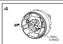
Secure fixture with screws and o-rings supplied - do not use power tools - screw by hand to prevent oring/gasket damage.
