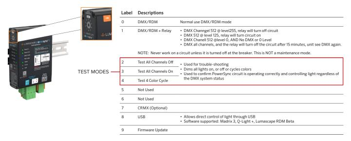
The LS6555 provides three (3) test modes for PowerSync luminaires. These require only connected luminaires and power, and no connected input signal. If an input signal is connected, the LS6555 will not respond to this signal in any of the modes below.
